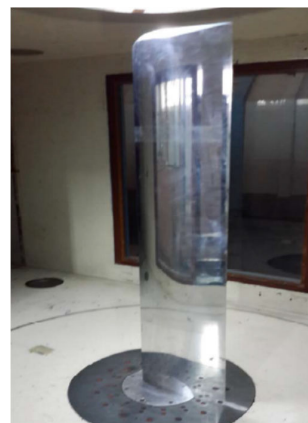
Fig. 3 Half model tested in IIUM-LSWT
