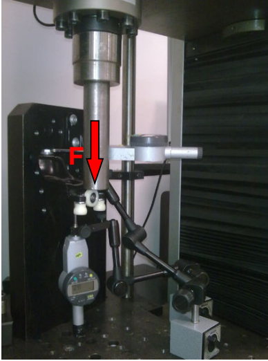
Fig. 12 Physical test set up for mechanism stiffness
