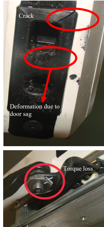
Fig. 13 Part fails from durability test [6]
