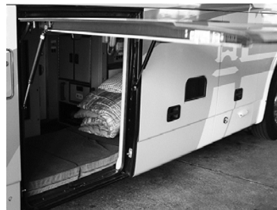
Fig. 7 Photograph of an example of driver's rest room in the bus cabin which is modified from the luggage hold
