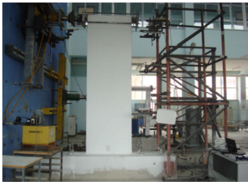
Fig. 5 The photograph of the test Setup, Loading System and Instrumentation of CSW
