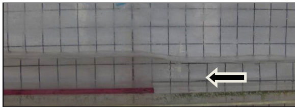
Fig. 13 Free-surface for F = 2.77 and B = 0.2
