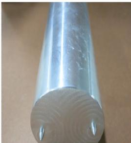
Fig. 6 The real horn made by aluminum
