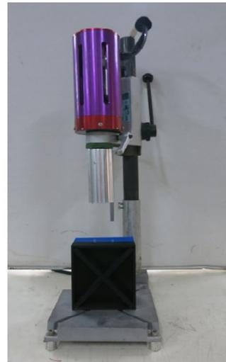
Fig. 8 Ultrasonic tube flanging specialized station
