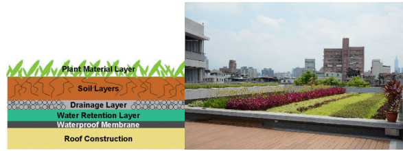
Fig. 2 The green roof configuration and environment images
