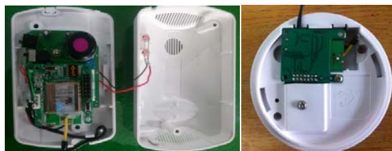
Fig. 5 CO and smoke detector with wireless module
