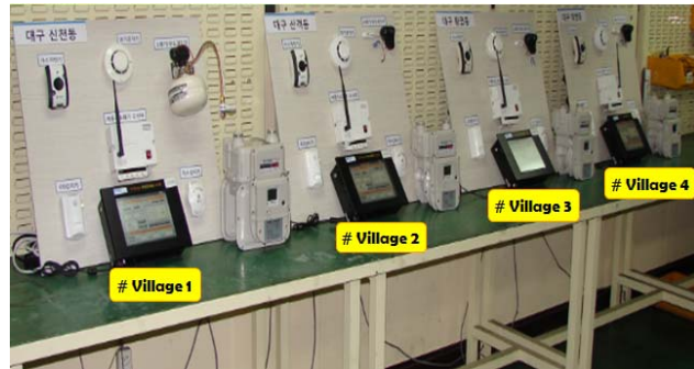
Fig. 14 Performance test of multiple monitoring systems
