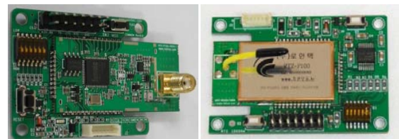
Fig. 1 Wireless modules with JN5139 microcontroller
