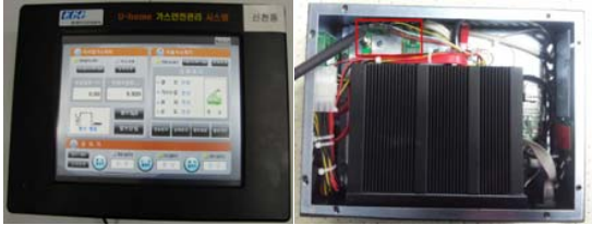
Fig. 6 Front and rear sides of a wall-pad with wireless module
