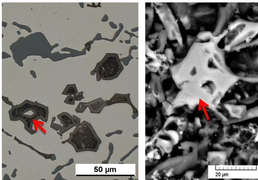
Fig. 6 The Fe-rich intermetallic phases  $Al_{15}(FeMnCr)_3Si_2$  in secondary AlSi9Cu3 cast alloy, as-cast state; (a)  $Al_{15}(FeMnCr)_3Si_2$  multi-component sludge; (b)  $Al_{15}(FeMnCr)_3Si_2$  multi-component sludge-SEM
