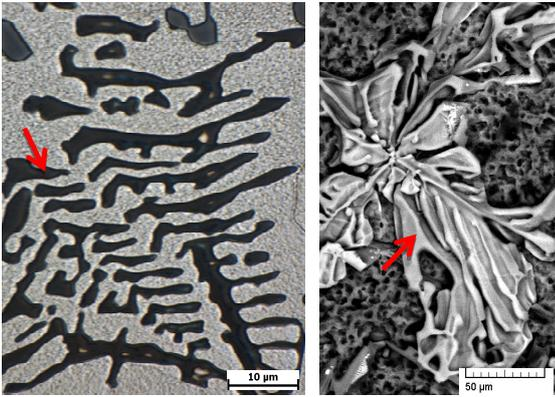
Fig. 5 The Fe-rich intermetallic phases  $Al_{15}(FeMn)_3Si_2$  in secondary AlSi9Cu3 cast alloy, as-cast state; (a)  $Al_{15}(FeMn)_3Si_2$  skeleton like; (b)  $Al_{15}(FeMn)_3Si_2$  skeleton like - SEM
