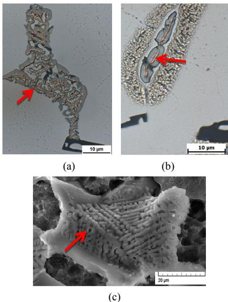
Fig. 3 The Cu-rich intermetallic phases in secondary AlSi9Cu3 cast alloy, as-cast state; (a) Al-Al<sub>2</sub>Cu-Si; (b)  $\text{Al}_2\text{Cu}$ ; (c) SEM-Al-Al<sub>2</sub>Cu-Si
