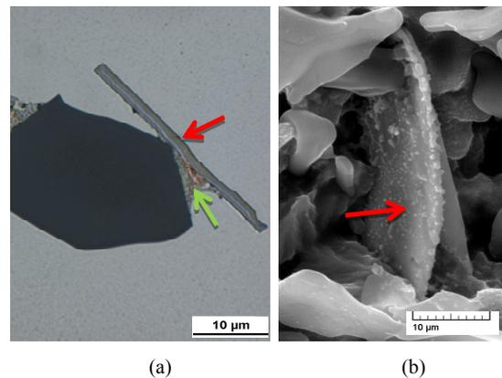
Fig. 4 The Fe-rich intermetallic phases  $\text{Al}_3\text{FeSi}$  in secondary AlSi9Cu3 cast alloy, as-cast state; (a)  $\text{Al}_3\text{FeSi}$  needles; (b)  $\text{Al}_3\text{FeSi}$  platelets- SEM
