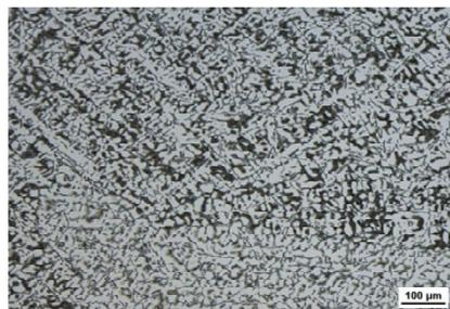
Fig. 1 The  $\alpha$ -phase in secondary AlSi9Cu3 cast alloy, as-cast state.
