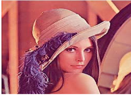
Fig. 6 (c) The 8x8 reconstructed fractal image of 1.009 bpp, 32.52 dB
