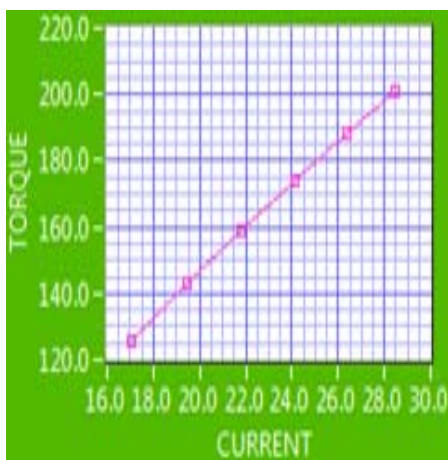
Fig. 4 Torque vs current characteristics of dc motor
