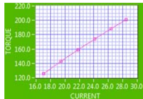
Fig. 5 Torque vs current characteristics of induction motor
