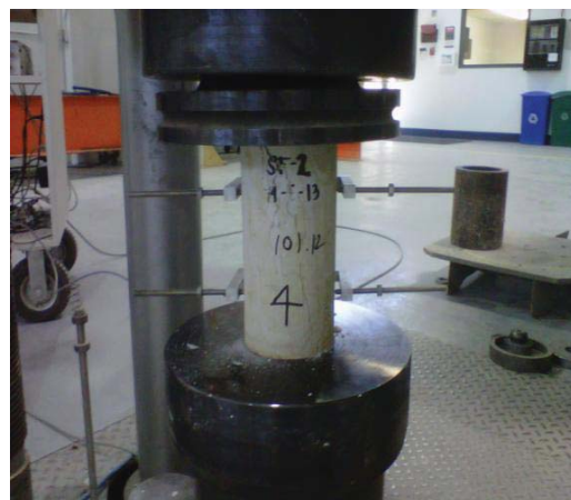
Fig. 5 Compressive Testing of the Overlay Material
