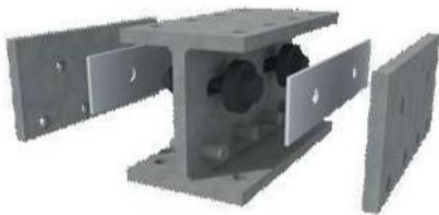
Fig. 8 Shear friction damper
