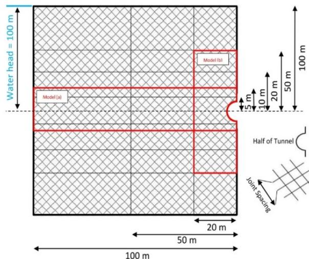
Fig. 1 Model geometry with extent of model domain *ME* for different model dimensions. For example, in model (a) of this figure, the horizontal model dimension (*ME h*) is 100 m and vertical model dimension (*ME v*) is 10 m and in model (b), these dimensions are 20 and 50 m, respectively
