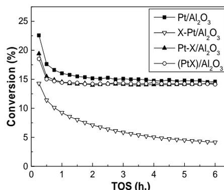
Fig. 3 Propane conversion with time on stream
