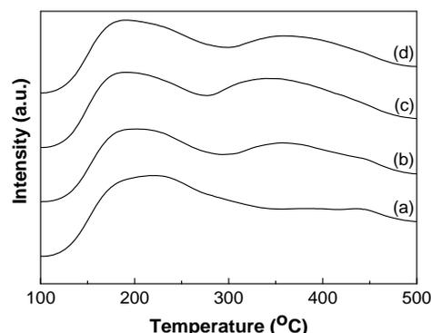
Fig. 1 NH<sub>3</sub>-TPD profiles of catalysts; (a) Pt/Al<sub>2</sub>O<sub>3</sub>, (b) X-Pt/Al<sub>2</sub>O<sub>3</sub>, (c) Pt-X/Al<sub>2</sub>O<sub>3</sub> and (d) (PtX)/Al<sub>2</sub>O<sub>3</sub>
