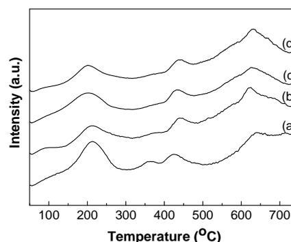
Fig. 2 TPR profiles of catalysts; (a) Pt/Al<sub>2</sub>O<sub>3</sub>, (b) X-Pt/Al<sub>2</sub>O<sub>3</sub>, (c) Pt-X/Al<sub>2</sub>O<sub>3</sub> and (d) (PtX)/Al<sub>2</sub>O<sub>3</sub>
