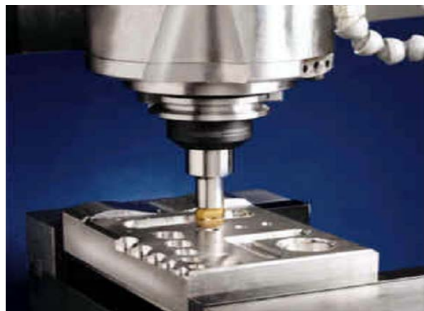
Fig. 1 End Milling Operation on D2 steel
