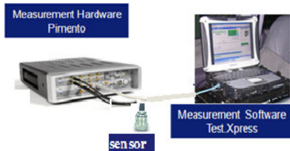
Fig. 4 Typical setup of transducer-data acquisition pair
