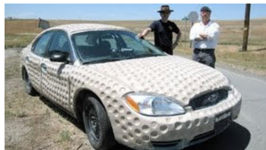
Fig. 2 The Mythbusters crew experimented with dimples on this Ford Taurus
