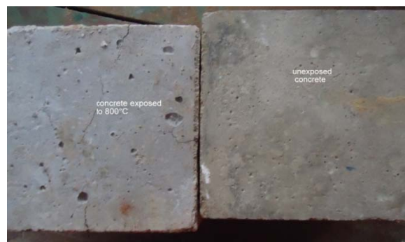
Fig. 2 Concrete exposed to 800°C
