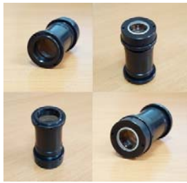
Fig. 2 Optical system of star tracker experimental model
