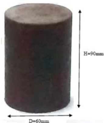
Fig. 2 Sample prepared; D= 60 & H= 90 mm
