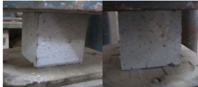
Fig. 2 Concrete specimens subjected to 400°C and 600°C
