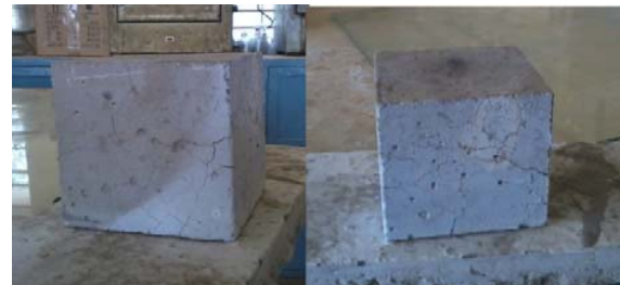
Fig. 3 Concrete specimens subjected to 800°C
