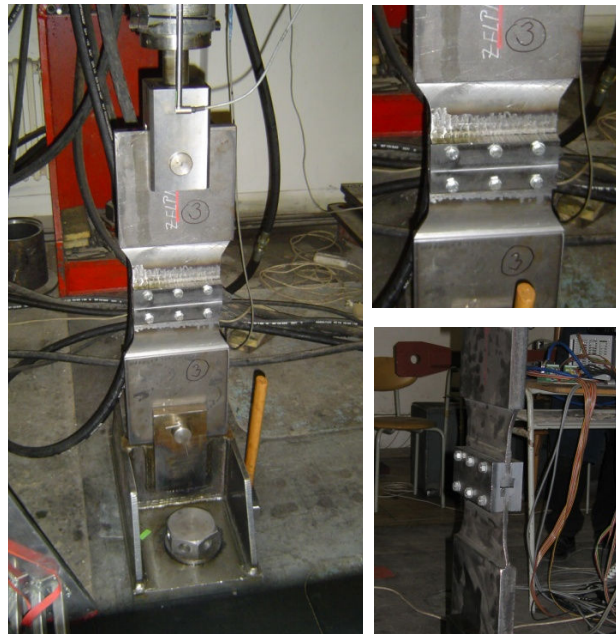
Fig. 4 Realization of cyclic loading tests
