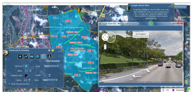
Fig. 4 Use interactively for proposing boreholes and seismic survey lines
