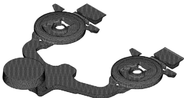
Fig. 4 Finite element model of a HPDC part cavity for two motorcycle fuel caps
