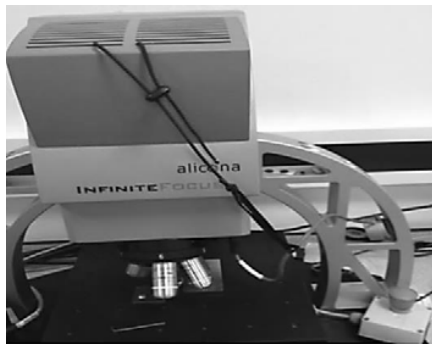
Fig. 10 3D wear measurements using alicona (INFINITE FOCUS)
