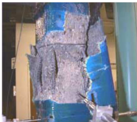
(b) Real cracks distribution [12]
