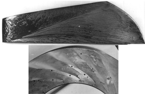
Fig. 4 Flow visualization in stage components Suction side of a 2D impeller blade, surge flow rate and flow separation zone in a vane diffuser
