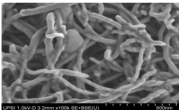
Fig. 8 FESEM images of MWCNTs-calix[8]arene with \text{Cd}^{2+}
