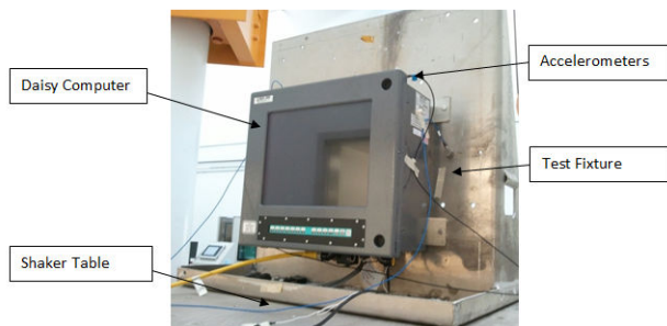
Fig. 3 Test setup for Daisy Data Displays computer
