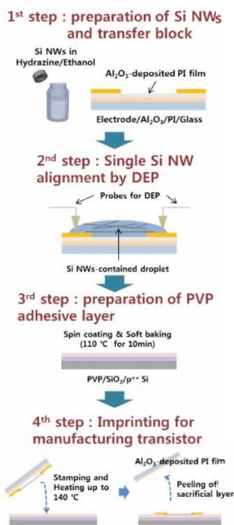
Fig. 1 The process flow sequence to imprinting and fabrication of circular Si NWs FET using \text{Al}_2\text{O}_3 layer as a sacrificial transfer layer
