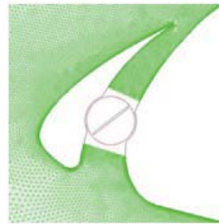
Fig. 5 Close up of mesh. Mesh in inner domain removed for clarity. Red line represents the interface between the rotating and stationary domain
