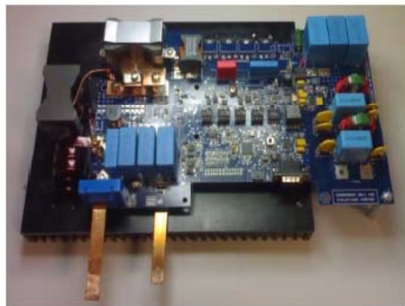
Fig. 3 1.5 KW Converter used for the design
