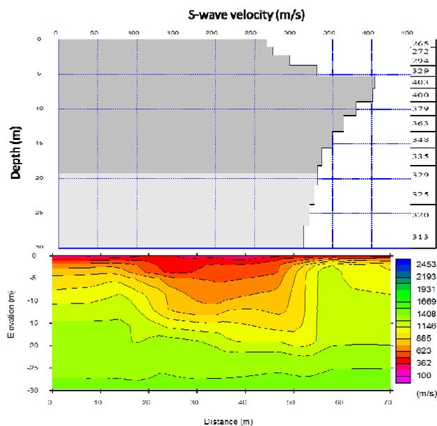
Fig. 2 Profile P wave velocity-depth model and velocity cross-section
