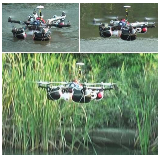
Fig. 10 Successful test of taking off of hexarotor from the water
