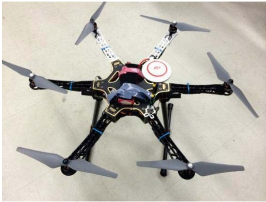
Fig. 1 Completely assembly of the DJI F550 Hexarotor
