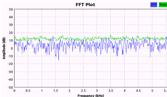
Fig. 9 Captured FM signal from .dat file
