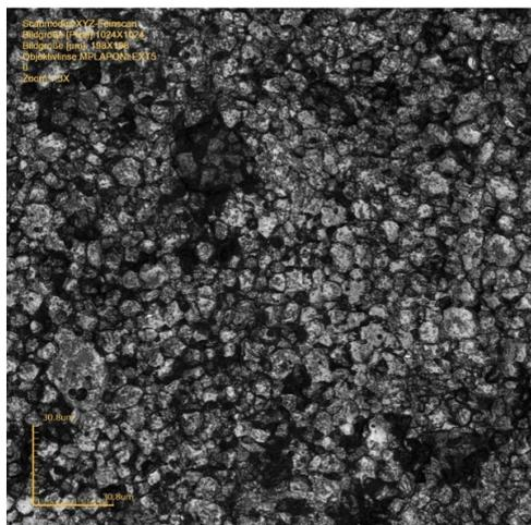
Fig. 5 CLSM of S2 magnet before corrosion (30 by 30 μm)
