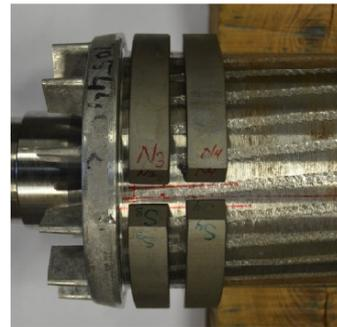
Fig. 3 Magnets attached to rotor without any protective coating on surface and left at room temperature for 7 days
