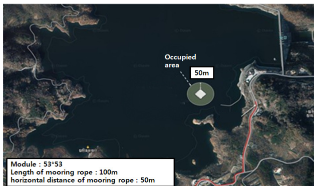
Fig. 2 Installation position of substantiation-plant
