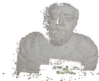
Fig. 6 CloudCompare output model using Poisson algorithm
