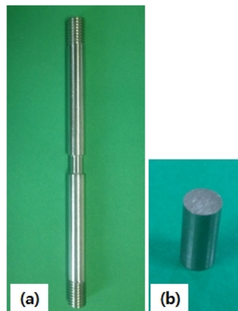
Fig. 3 Appearance of tensile (a) and compressive (b) specimen used in this study
