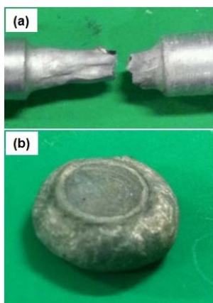
Fig. 6 Appearances of specimens after tensile (a) and compression tests conducted at temperatures of 1200°C
