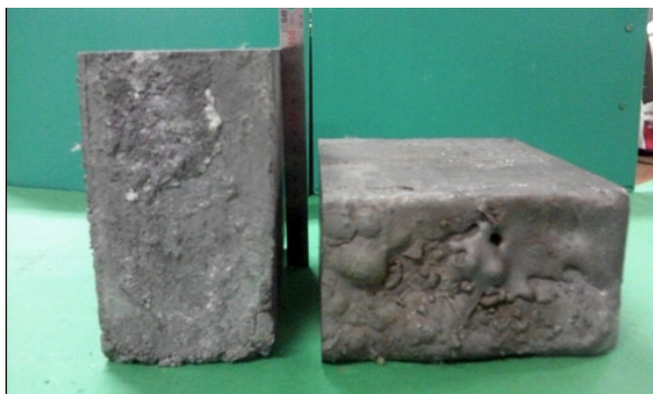
Fig. 2 Appearance of the Fe-20Cr-5Al ferritic stainless steel used in this study
