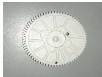
Fig. 2 (a) Plastic, 70 teeth, 3.5cm diameter gear
