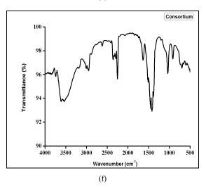
Fig. 1 (a)-(f) FT IR of Carbendazim, Endosulfan and Imidacloprid degraded by bacterial consortia after degradation
