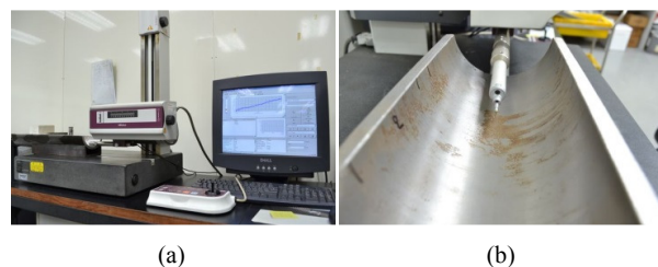
Fig. 2 (a) Surface roughness measuring system (b) Surface roughness measuring probe and tested workpiece
