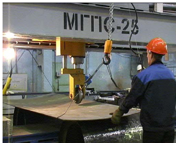
Fig. 4 Bending plate with MGPS-25 machine
