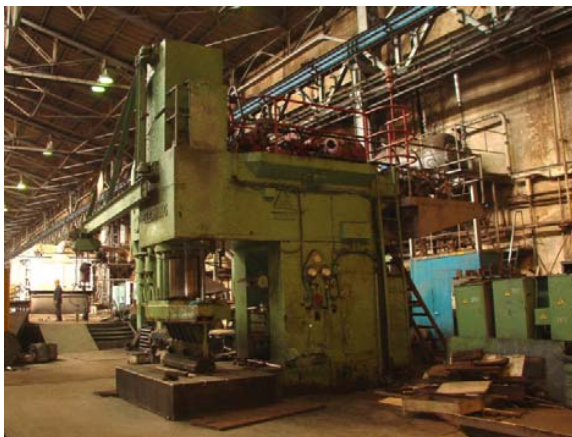
Fig. 1 Press "Clearing", 3500 kN (350t) capacity
