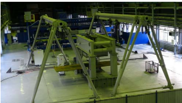
Fig. 6 Bending plate with MGPS-100 machine
