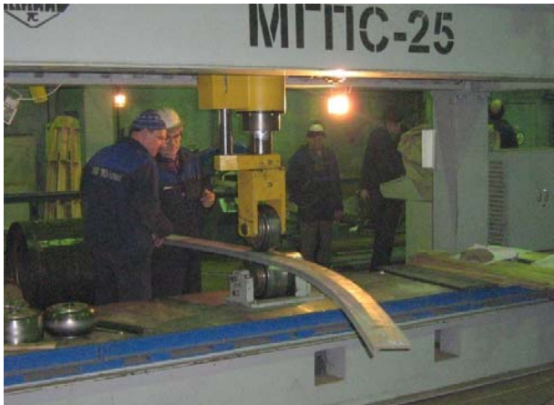
Fig. 5 Bending profile with MGPS-25
