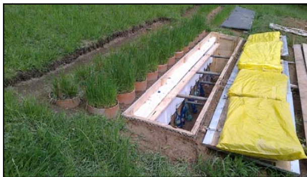
Fig. 2 Detail of the lysimetric experiment and control shaft
