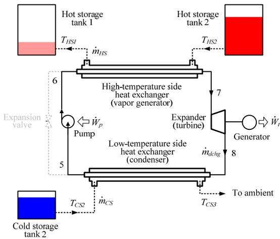
Fig. 2 Schematic diagram of discharging process
