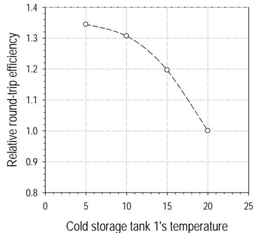
Fig. 3 Performance variation of the TEES according to the changes in the temperature of the cold storage tank
