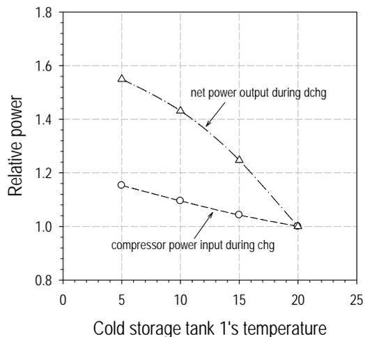
Fig. 4 Relative power variation according to the changes in the temperature of the cold storage tank
