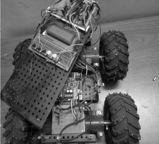
Fig. 14 H/W wiring implementation of the designed control system
