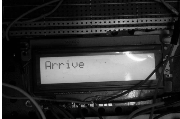
Fig. 16 Station arrival indication
