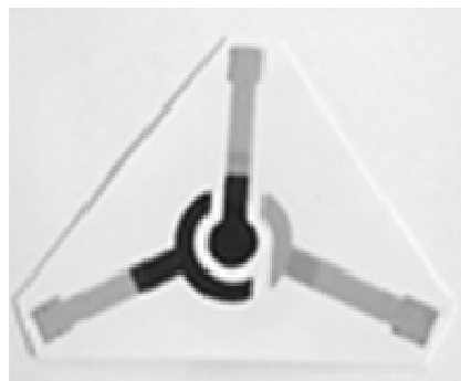
Fig. 1 The screen printed carbon electrode
