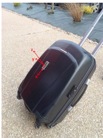
Fig. 4 Slam Stick USB Key on the Luggage
